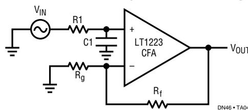
It is very common to limit the bandwidth of an op amp by putting a small capacitor in parallel with  $R_f$ . This works with all unity gain stable op amps; DO NOT PUT A SMALL CAPACITOR FROM THE INVERTING INPUT OF A CURRENT FEEDBACK AMPLIFIER TO ANYWHERE, ESPECIALLY NOT TO THE OUTPUT. The capacitor on
