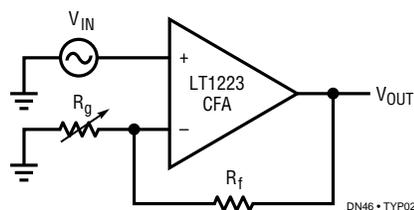
With a standard op amp you can vary the gain of the amplifier with either  $R_f$  or  $R_g$ . The only real restriction on the values is the loading affect the resistors have on the amplifier output. With a current feedback amplifier the value of  $R_f$  should not be varied. Do not make  $R_f$  the variable resistor or the bandwidth will be reduced at maximum gain and the circuit will oscillate when  $R_f$  is very small.
