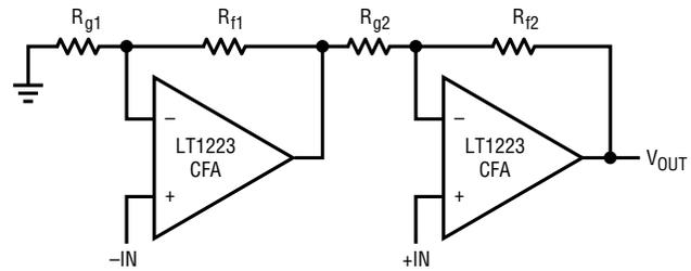
TRIM  $R_{g2}$  FOR GAIN, THEN TRIM  $R_{g1}$  FOR CMRR. VOLTAGE GAIN,  $G$ , IS  $V_{OUT}$  DIVIDED BY DIFFERENCE BETWEEN  $+IN$  AND  $-IN$ .
