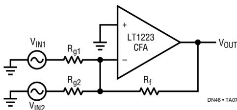
There is no  $I_{OS}$  spec on current feedback amplifiers because there is no correlation between the two input bias currents. Therefore we will not improve the DC accuracy of the inverting amplifier by putting an extra resistor in the non-inverting input. This is also true of input bias current canceled op amps where the  $I_{OS}$  spec is the same as the  $I_B$  spec, such as the LT1220.
