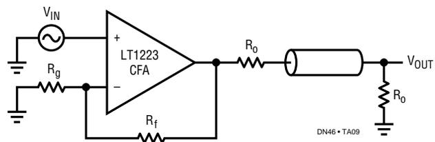
The cable driver circuit is the same for both types of amplifiers. But because most op amps do not have enough output drive current, they are not often used for heavy loads like cables. When driving a cable it is important to properly terminate both ends if even modest high frequency performance is required. The additional advantage of this is that it isolates the capacitive load of the cable from the amplifier so it can operate at maximum bandwidth.
